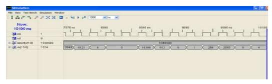
The above shows the output snap of Accessing password. In order to generate Accessing password control signal 'rst' should be set to '0' and input taken in the above step is '1645550' finally yielded output is '2048'. Accessing password is used to access the data in tag authentically. If authentication success tag will send information to reader else mismatch occurs between the tag and the reader.
